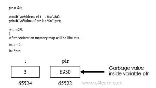
after Assigning the address of variable to pointer, i.e after the execution of this statement – ptr = &i;
