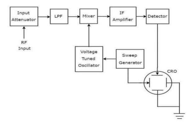
The working of superheterodyne spectrum analyzer is mentioned below.
