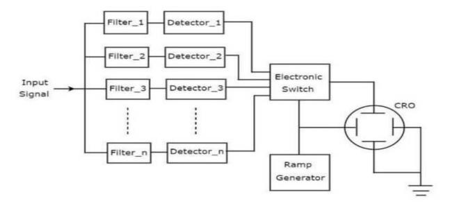
The working of filter bank spectrum analyzer is mentioned below.
