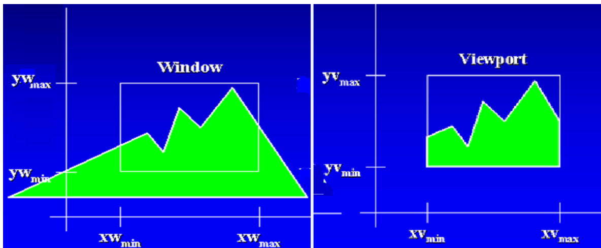
Figure 4-2 A clipping window and associated viewport, specified as rectangles aligned with the coordinate axis.
