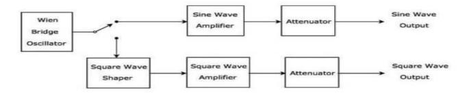
The above block diagram consists of mainly **two paths**. Those are upper path and lower path. Upper path is used to produce AF sine wave and the lower
